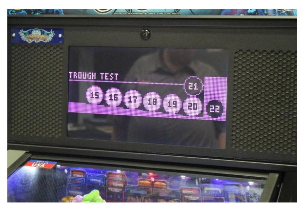
6. As the balls come down the playfield, pick them up and place in a secure location. Once all balls have been ejected from trough, it is safe to lift your playfield or move your pinball machine.
