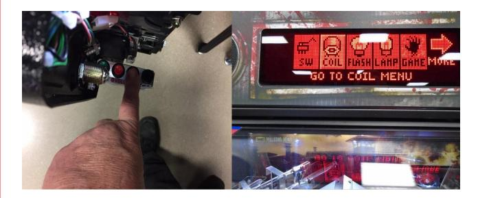
8. Press the "Menu" button to enter the coil test.
